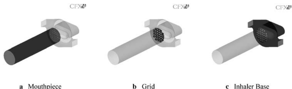
Fig. 1. Schematic of the different sections of the Aerolizer ® used when determining the frequency and location of particle–device impactions.
